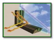
Double-pane glass can help reduce the risk of fracture or collapse during an extreme wildfire. Tempered glass is the most effective. For skylights, glass is more fire resistant than plastic or fiberglass.
